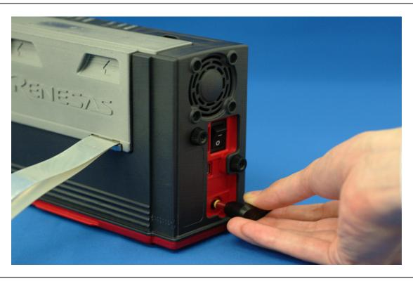
Figure 2.5 Connecting the emulator power supply
